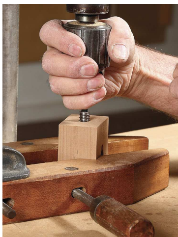
Mortise for the pressure pad. To cut the square mortise, go halfway through from one face, flip the head over, and finish the cut. A stop block ensures perfect alignment.
