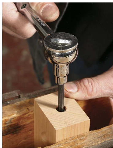
A hole for the beam. Again using the L-shaped fence to steady the head, drill completely through from one side, using a piece of MDF beneath to prevent blowout.
