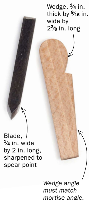
Make the wedge. A simple jig, which holds the blank at the correct angle, ensures that the wedge has the same angle as the mortise in the beam.
