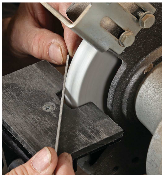
The blade is easy. Van Dyke uses a \frac{1}{4} -in. marking knife from Hock Tools for the gauge's blade, cutting off the first 2 in. at the grinder.
