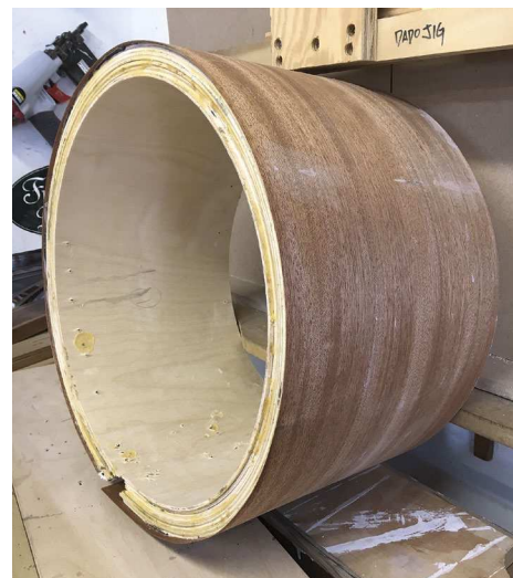
Veneer on the drumhead. With the substrate cured, Strout applied mahogany veneer to the exterior. Later, he cut the drumhead to width and cut out the bottom segment of the circle.
