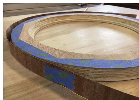
Decorating the door frame. Having already veneered the back of the drumhead door frame, Strout wraps veneer around the perimeter. Last, he'll veneer the face of the frame, using wedge-shaped pieces to create radiating grain.
