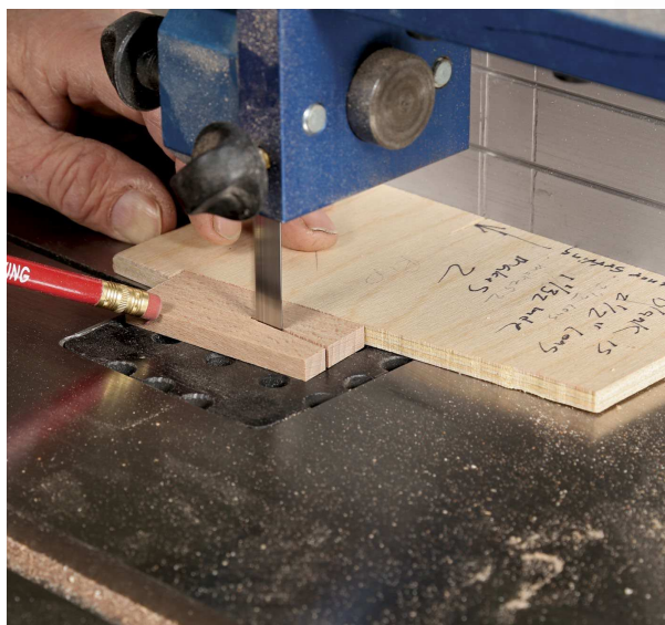
Make the wedge. A simple jig, which holds the blank at the correct angle, ensures that the wedge has the same angle as the mortise in the beam.
