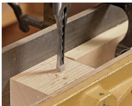
Mortise for the pressure pad. To cut the square mortise, go halfway through from one face, flip the head over, and finish the cut. A stop block ensures perfect alignment.
