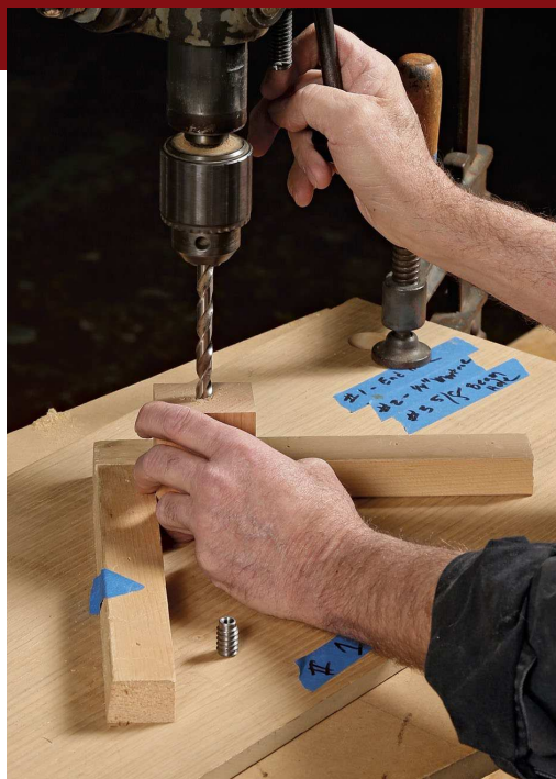
Drill for the threaded insert. Centered in one end, the hole extends halfway through the head. To steady the head during drilling, Van Dyke presses it into the corner of a right-angle fence.
