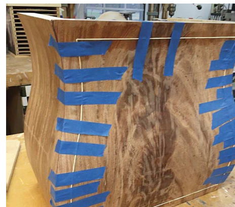
String clamp. With the base miters glued up, Strout used painter's tape as a clamp while he inlaid holly stringing into the crotch mahogany veneer.
