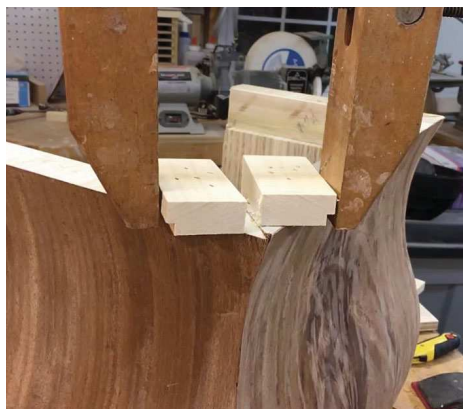
Tight squeeze. After veneering the curves and cutting the miters, Strout glued up using hand-screw clamps and clamping blocks to close the joints, then added band clamps.
