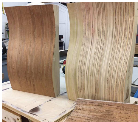
Stacked and shaped. Strout shaped the bombé base by bandsawing pieces of plywood to rough shape, face-gluing them, and then pattern-routing one from the next.
