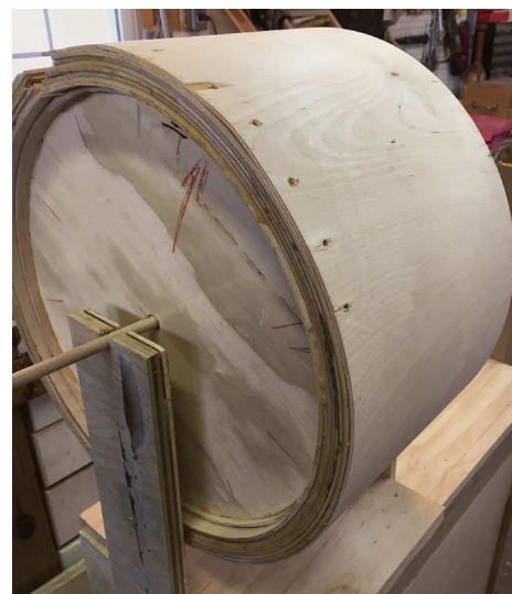
Circular assembly. To create the drumhead, Strout built a cylindrical form and laminated eight sheets of \frac{1}{8} -in.-thick bending ply around it, gluing them one at a time.
